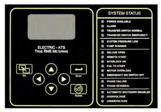
**Description**—Firetrol® FTA1300 Wye-Delta, Open Transition Starting Fire Pump Controllers are used with deltawound squirrel cage motors. FTA1300 controllers are of the open circuit transition type in which the motor circuit is opened during the transition from start to run. The controller monitors, displays and records fire pump system information.
